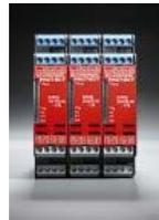
The PROTECT SRB 101-Ex (one safety release) and SRB 200 (two safety release) series are suitable for use in Ex zones. There are variants with monitored reset function (trailing edge) as well as with automatic or manual reset function. All these versions have a stop 0 safety release and optionally can be supplied with cross-wire short detection.
